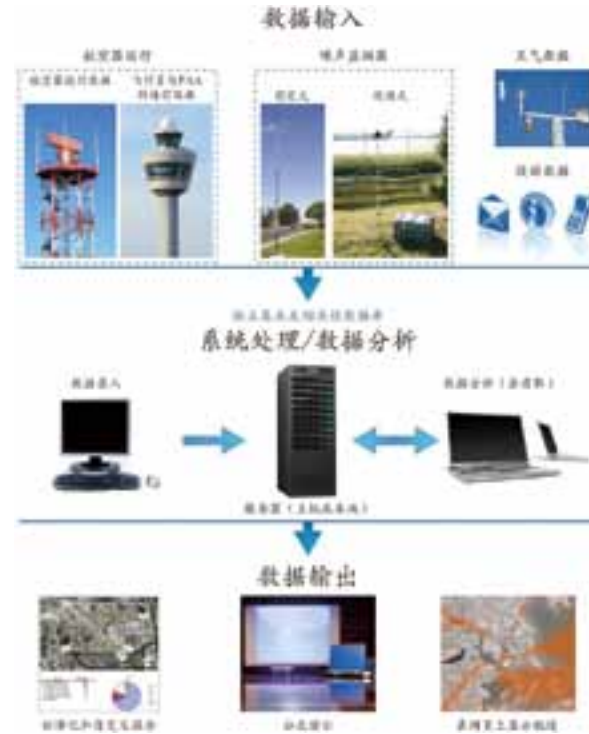
Below figure shows the work flow of noise monitoring software/hardware 下图为噪声监测软件硬件工作原理
