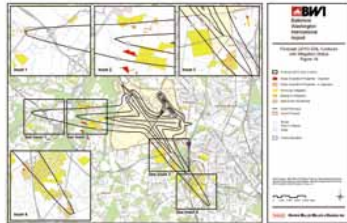
Below figure is the noise contour of Baltimore airport mapped according to the noise measurement 下图为根据噪声测量结果而绘制的美国巴尔的摩机场噪声等值线图
