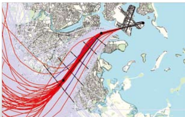
This figure compares flights using the improved departure procedure (red) against flights flown with the original procedure.
