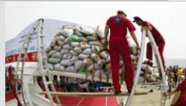
Zhuhai Jon members pile sandbags onto the composite wing to test its strength. Even with a load of 1800 kg of sandbags, the wing needed additional force before it finally broke.
